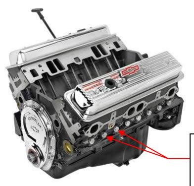
Install a UMSS engine seal through these two cylinder head bolts. Record the seal serial number on the checklist
