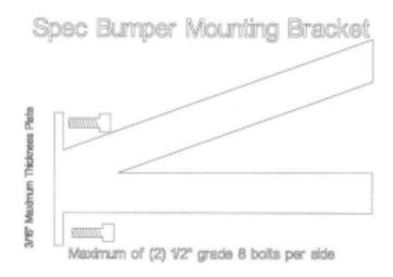
(1)Bracket per side of the car. Wrap around bars may circle around and be welded to the frame horn. No other bracing is allowed. Mounting bracket must also be made of  $1 \frac{1}{2}$  x .095 round tubing
